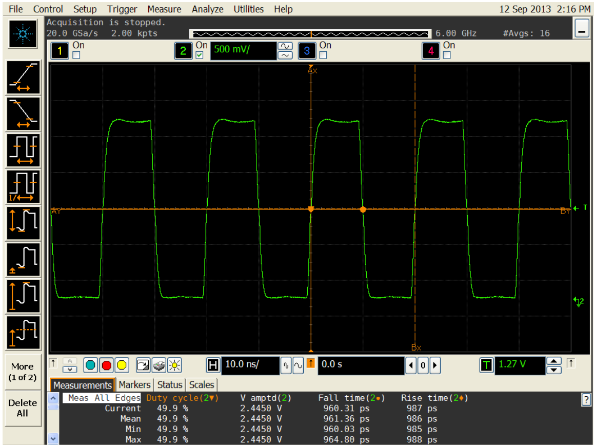
Figure 2. Duty cycle, Rise/Fall time and Amplitude 2.5V
