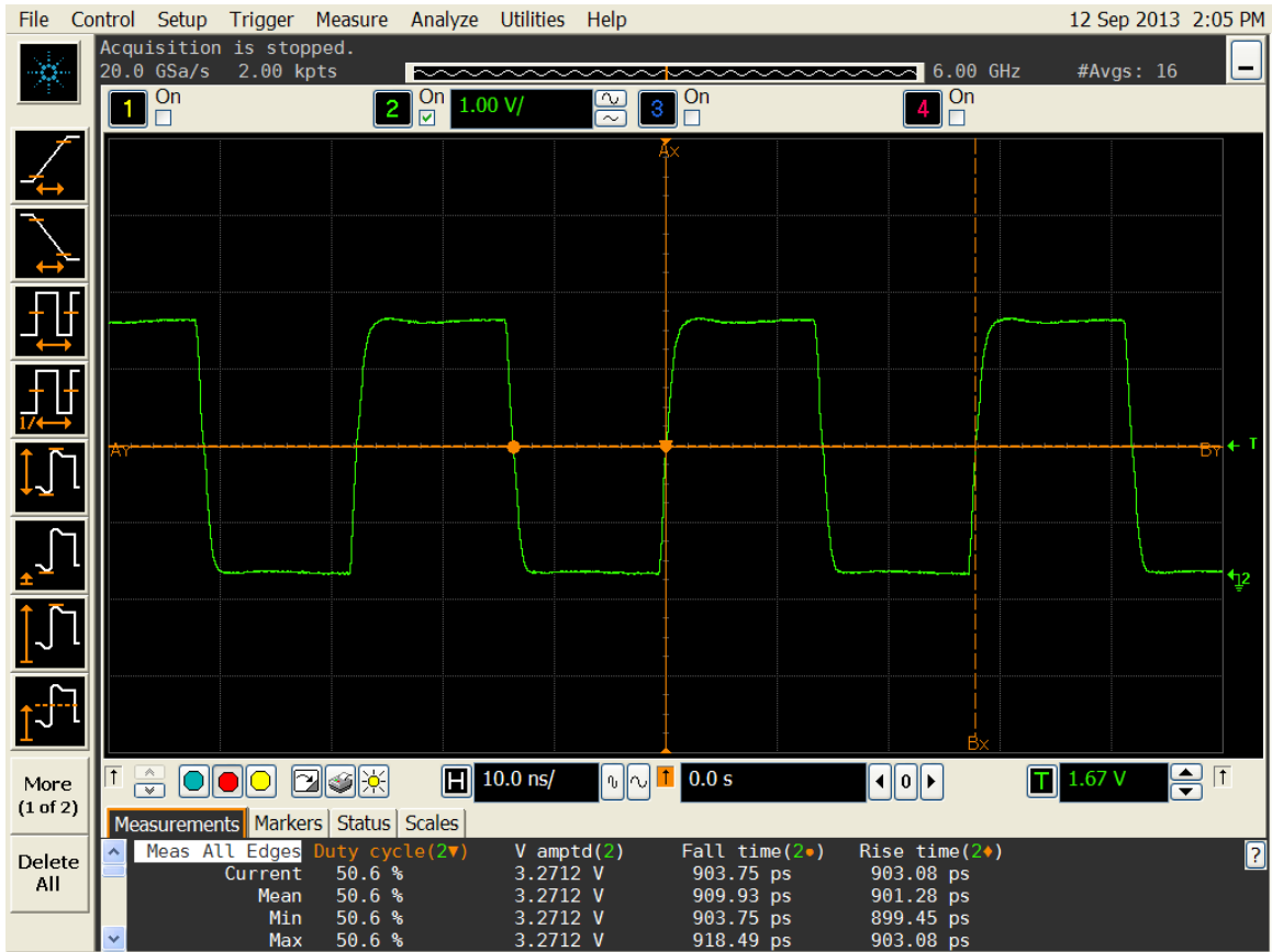
Figure 5. Duty cycle, Rise/Fall time and Amplitude 3.3V
