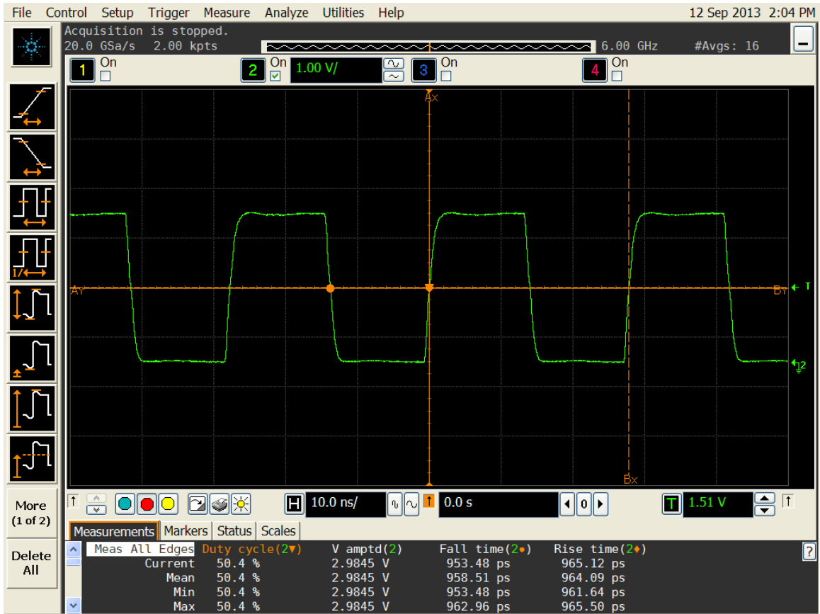
Figure 4. Duty cycle, Rise/Fall time and Amplitude 3.0V
