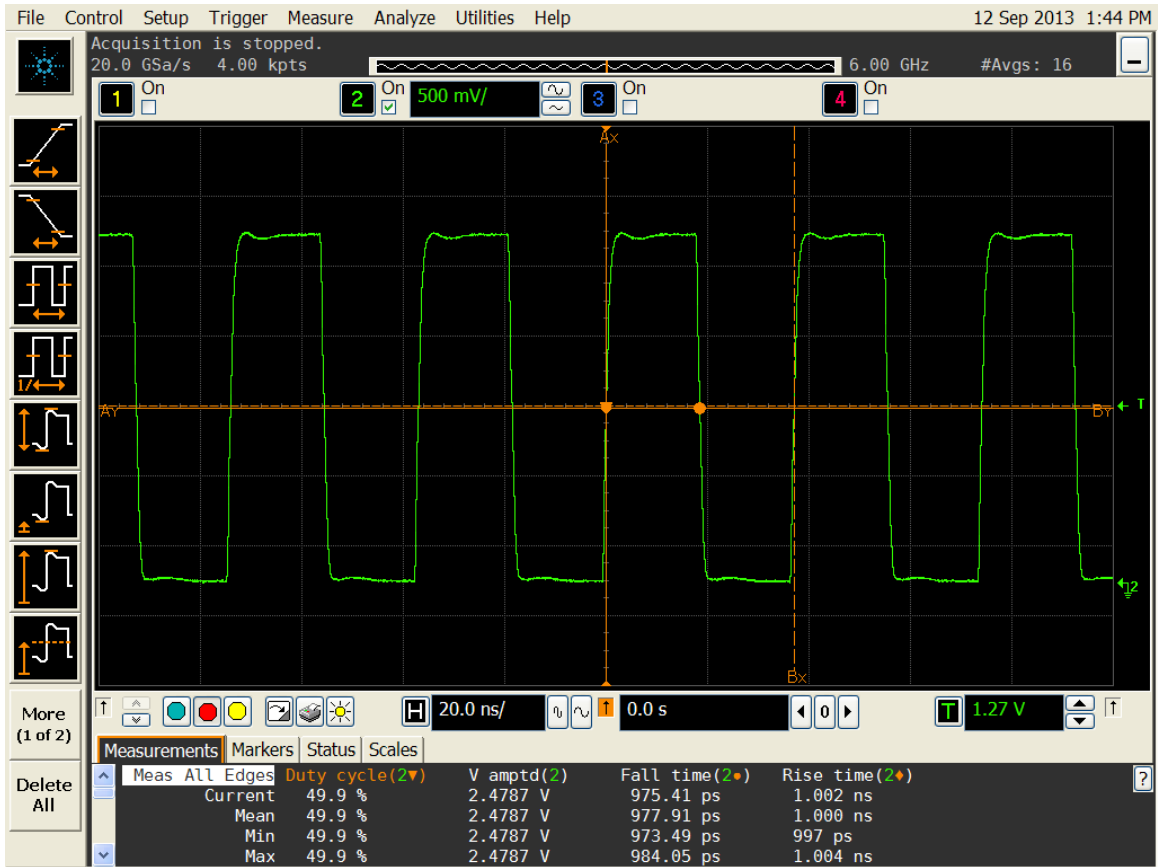
Figure 2. Duty cycle, Rise/Fall time and Amplitude 2.5V
