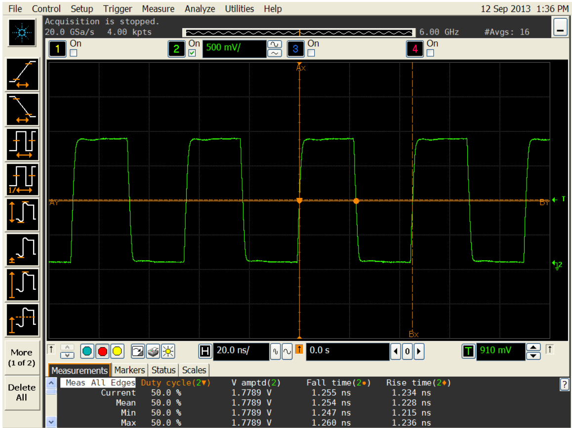
Figure 1. Duty cycle, Rise/Fall time and Amplitude 1.8V
