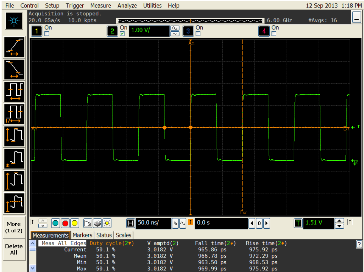
Figure 4. Duty cycle, Rise/Fall time and Amplitude 3.0V
