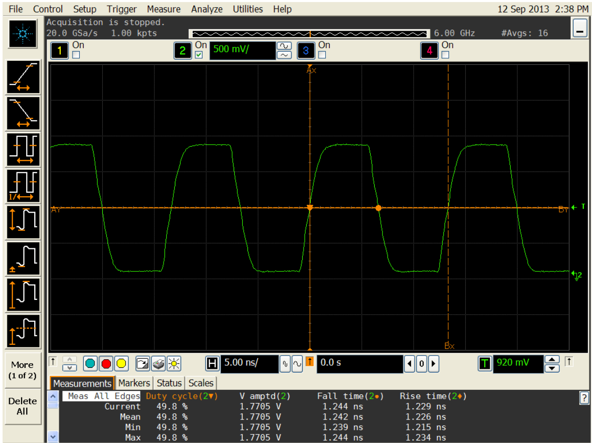
Figure 1. Duty cycle, Rise/Fall time and Amplitude 1.8V
