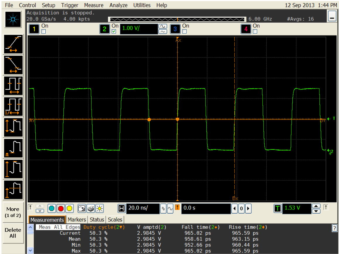
Figure 4. Duty cycle, Rise/Fall time and Amplitude 3.0V
