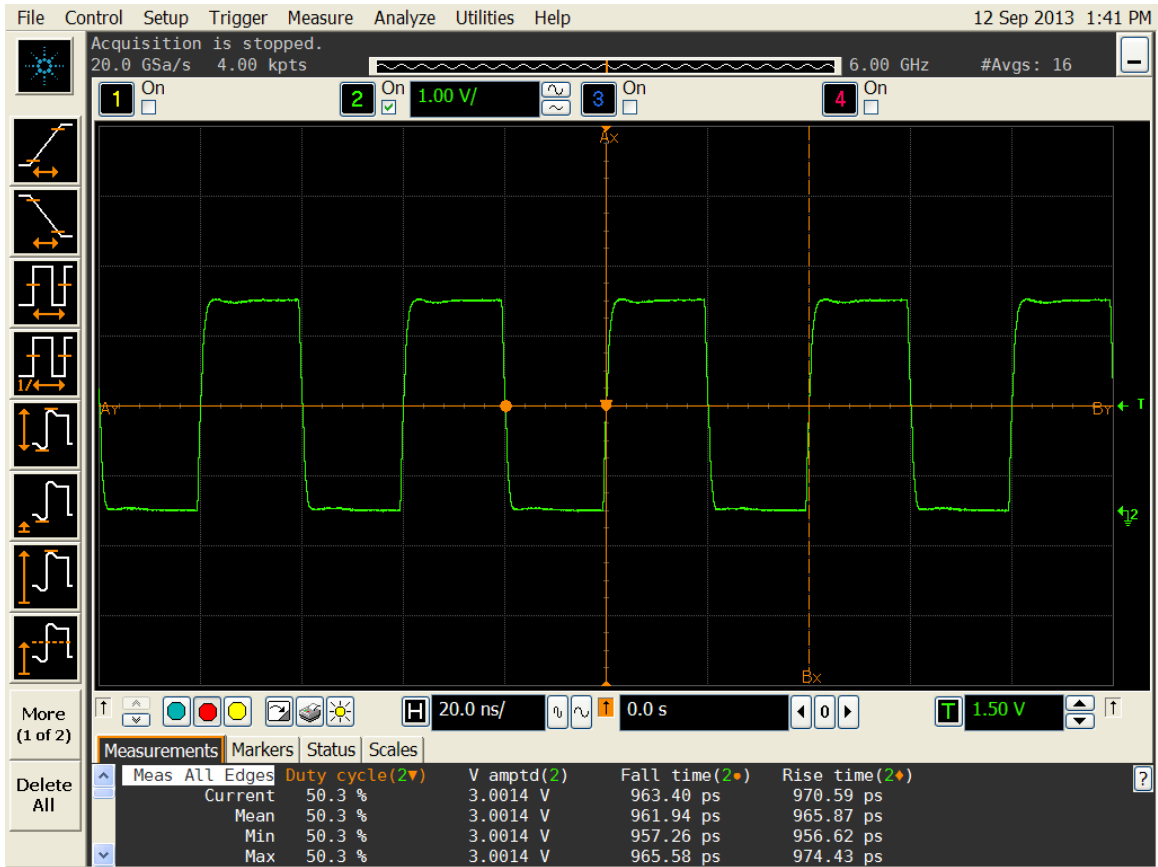
Figure 4. Duty cycle, Rise/Fall time and Amplitude 3.0V
