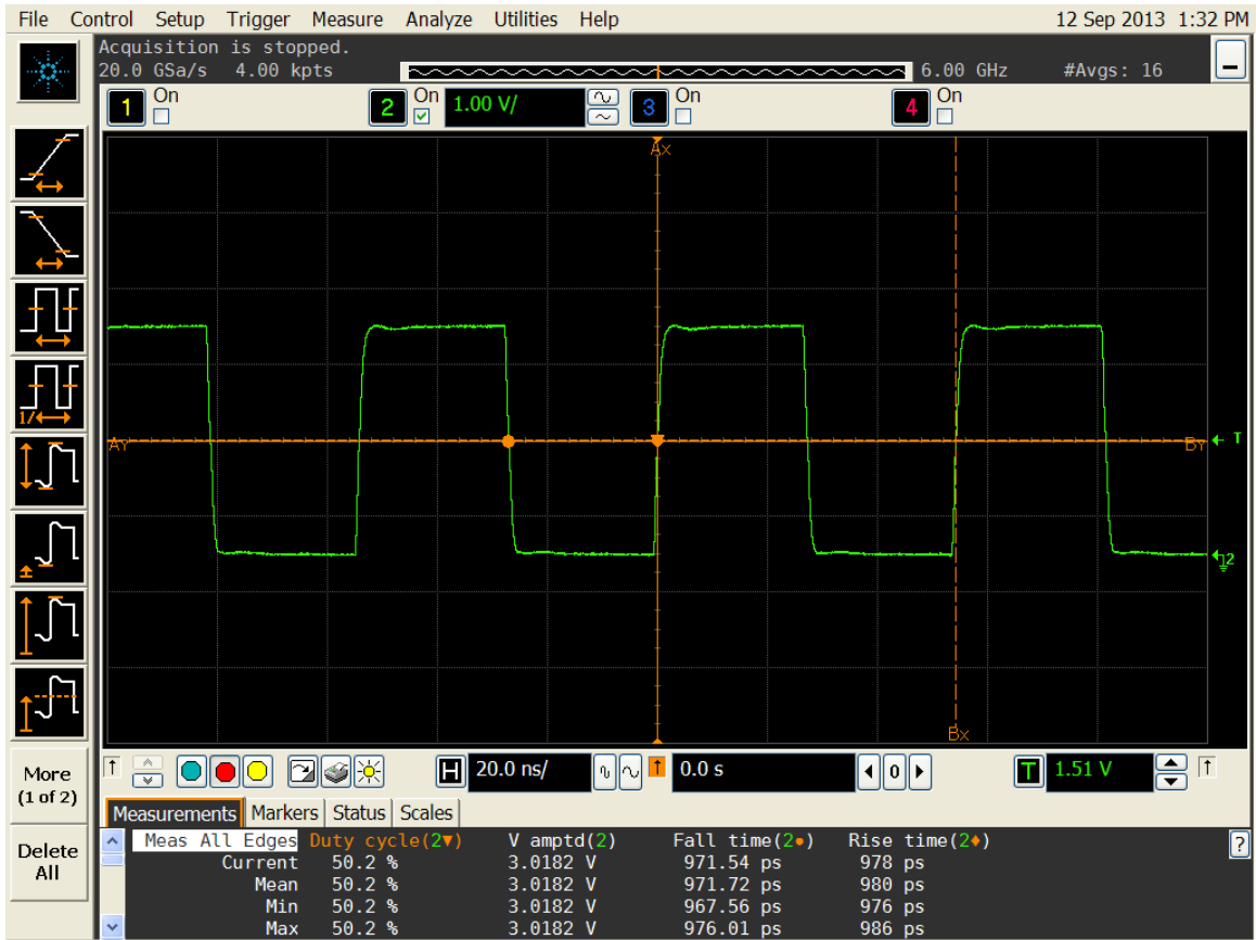
Figure 4. Duty cycle, Rise/Fall time and Amplitude 3.0V
