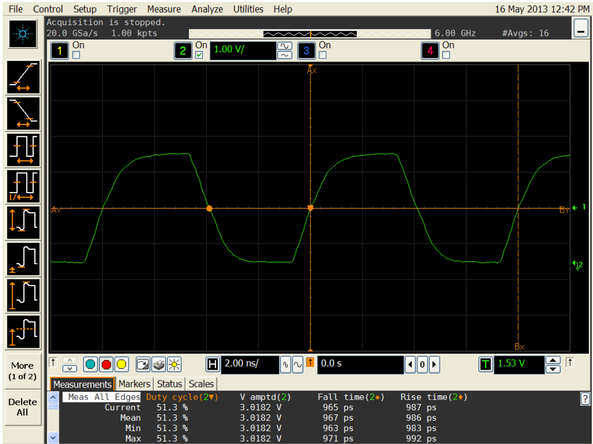
Figure 4. Duty cycle, Rise/Fall time and Amplitude 3.0V
