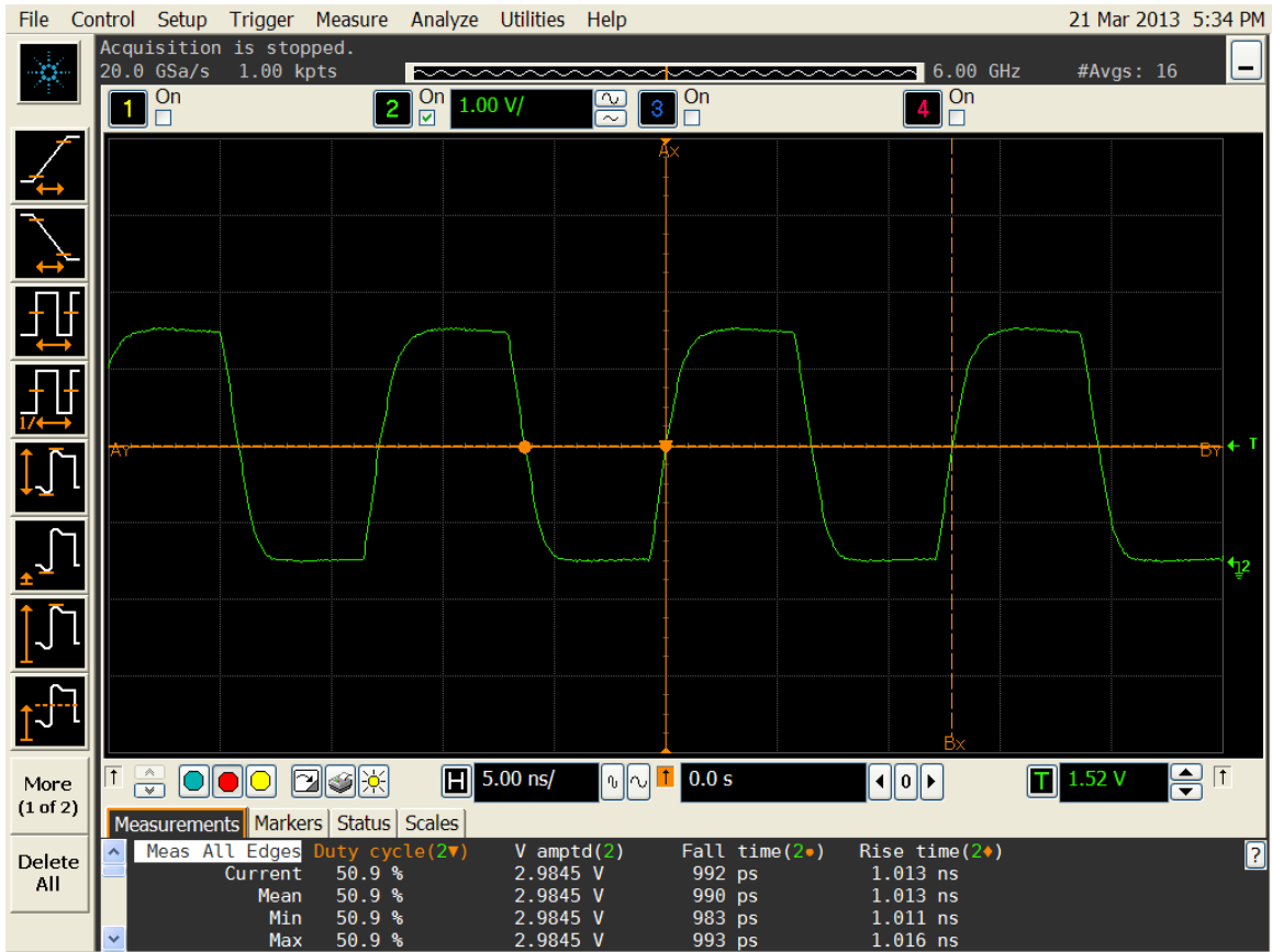
Figure 4. Duty cycle, Rise/Fall time and Amplitude 3.0V
