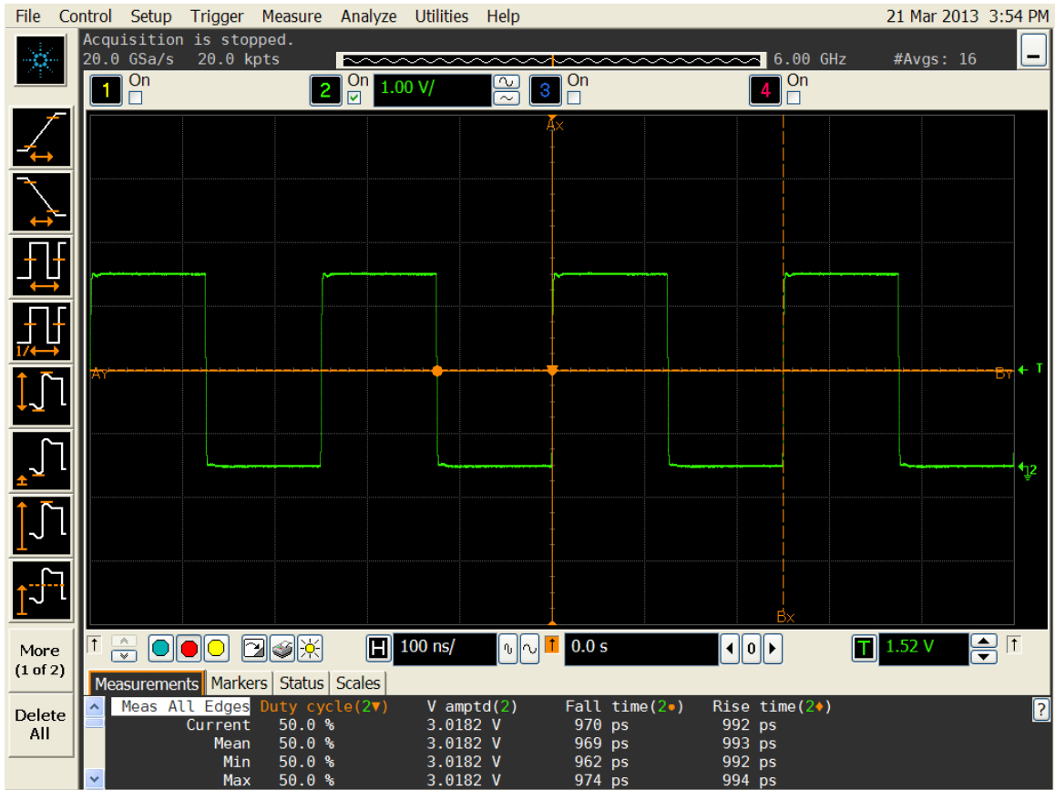
Figure 4. Duty cycle, Rise/Fall time and Amplitude 3.0V
