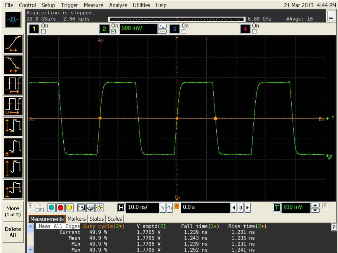
Figure 1. Duty cycle, Rise/Fall time and Amplitude 1.8V
