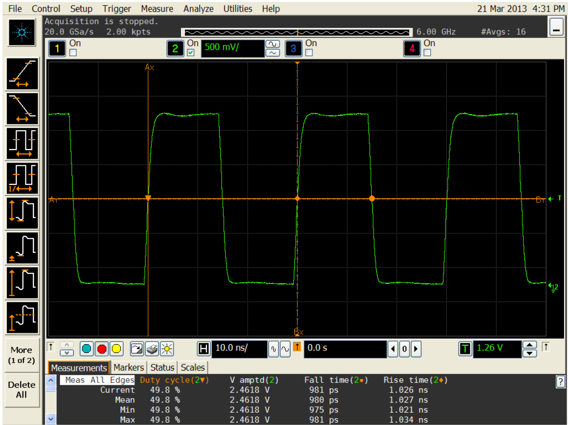
Figure 2. Duty cycle, Rise/Fall time and Amplitude 2.5V
