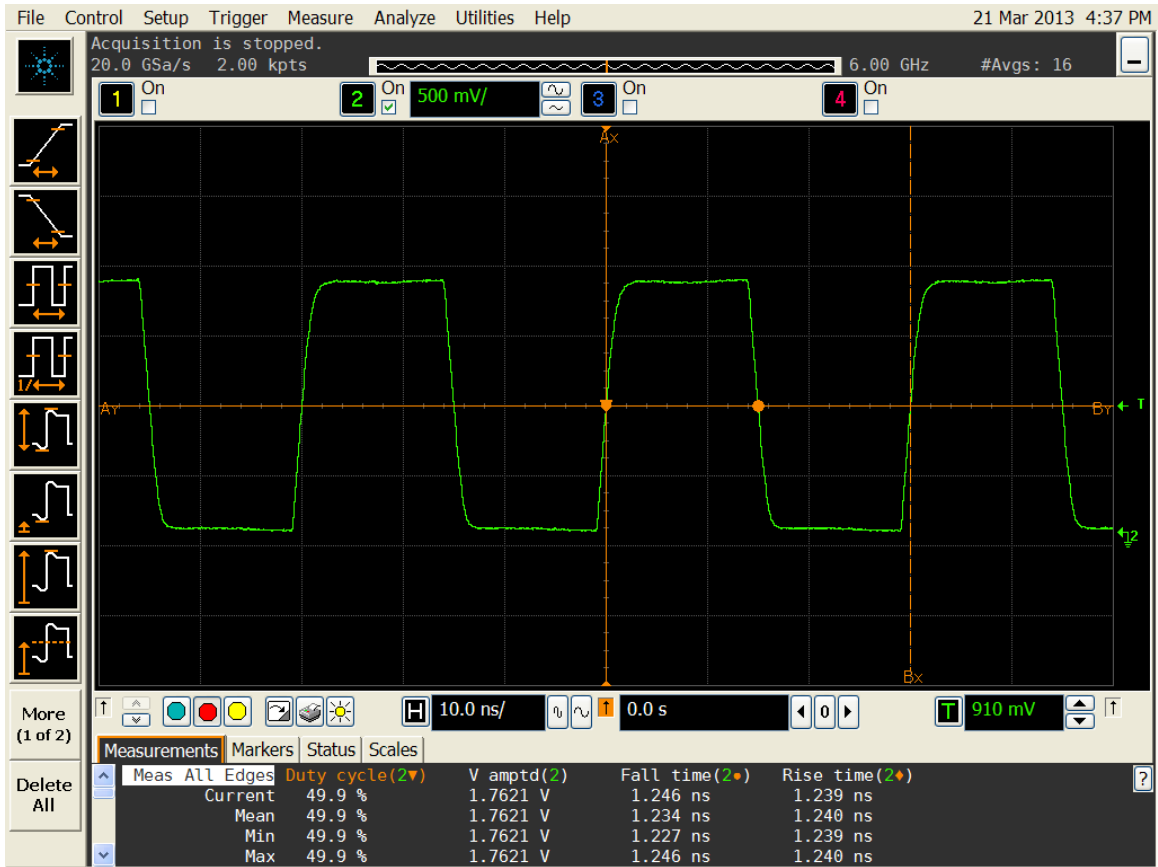
Figure 1. Duty cycle, Rise/Fall time and Amplitude 1.8V
