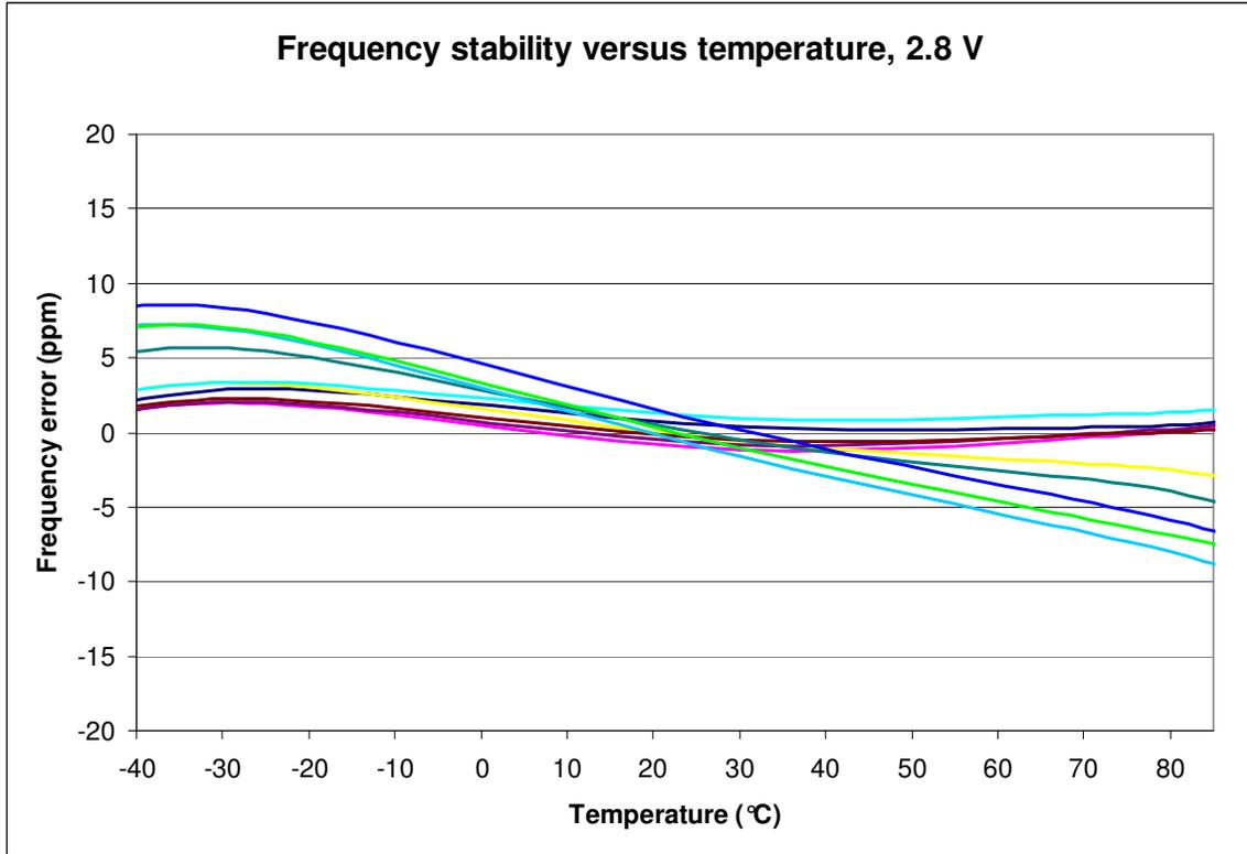
Figure 8. Frequency stability versus temperature, 2.8 V
