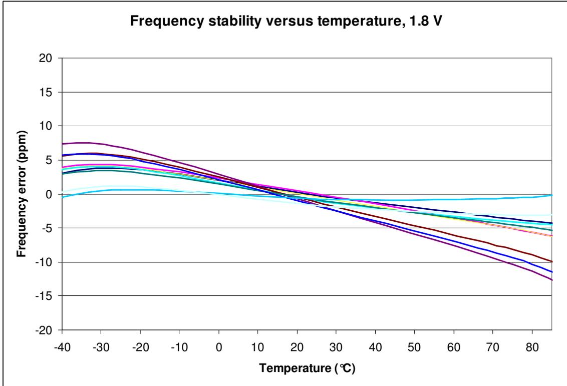
Figure 6. Frequency stability\* versus temperature, 1.8 V
