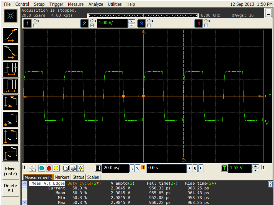
Figure 4. Duty cycle, Rise/Fall time and Amplitude 3.0V
