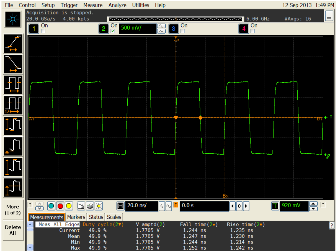
Figure 1. Duty cycle, Rise/Fall time and Amplitude 1.8V
