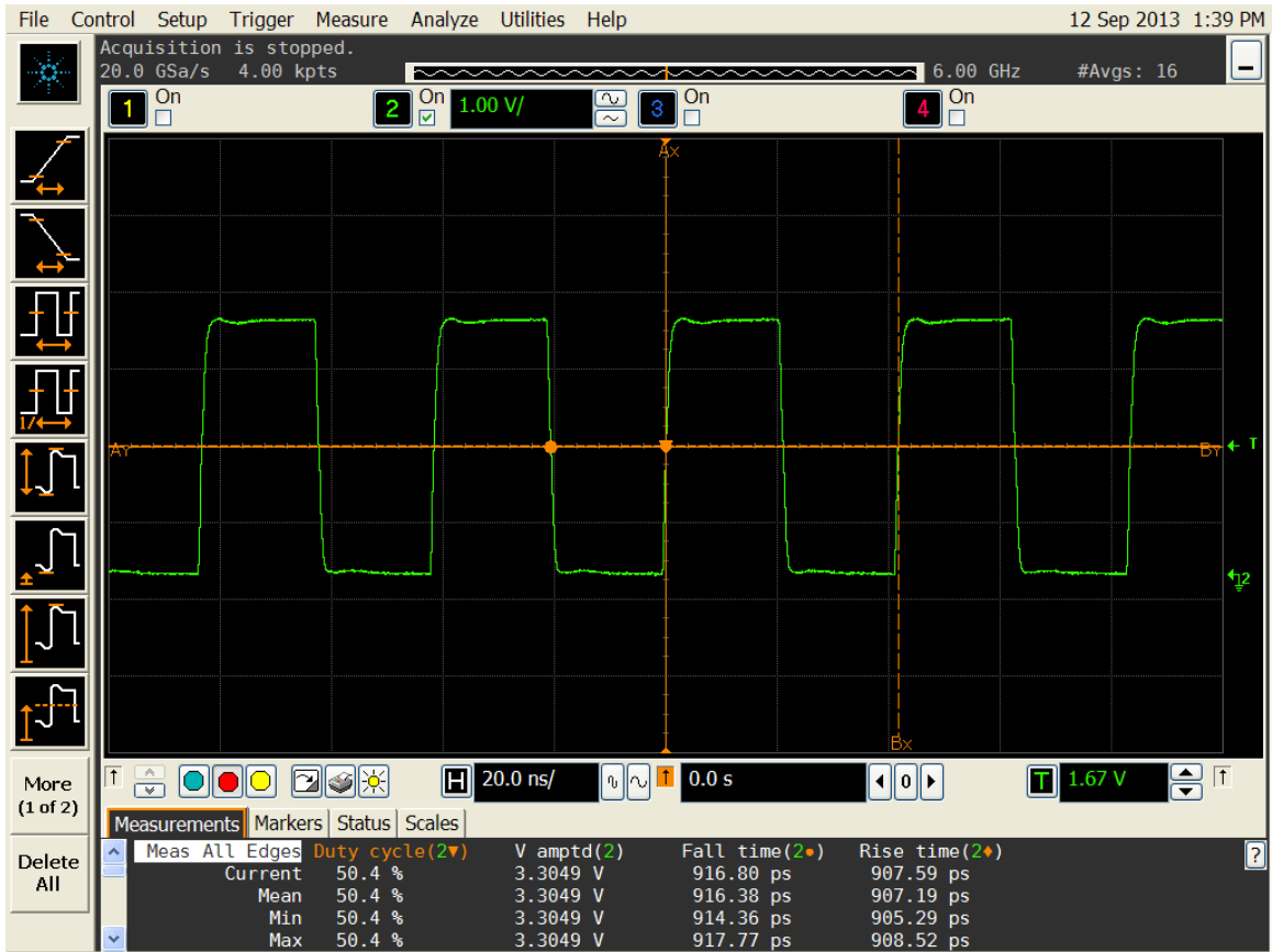
Figure 5. Duty cycle, Rise/Fall time and Amplitude 3.3V
