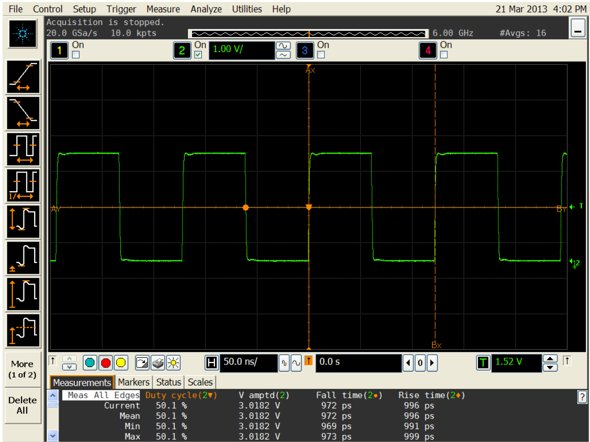
Figure 4. Duty cycle, Rise/Fall time and Amplitude 3.0V
