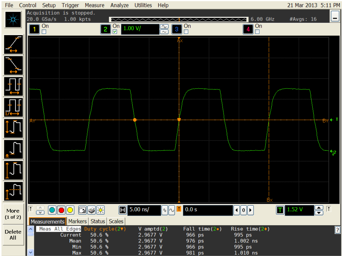
Figure 4. Duty cycle, Rise/Fall time and Amplitude 3.0V
