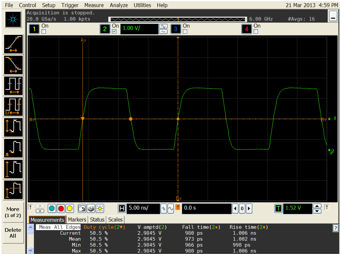
Figure 4. Duty cycle, Rise/Fall time and Amplitude 3.0V
