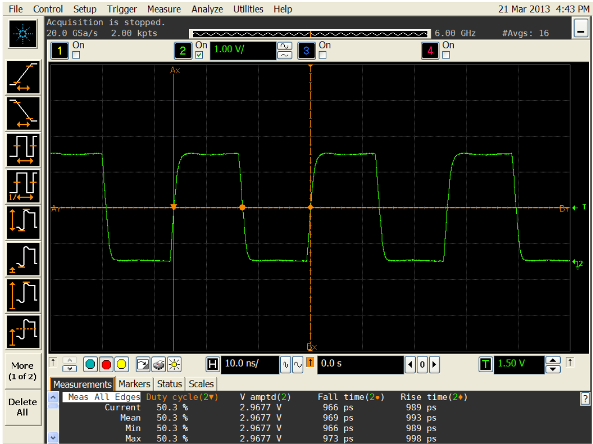
Figure 4. Duty cycle, Rise/Fall time and Amplitude 3.0V
