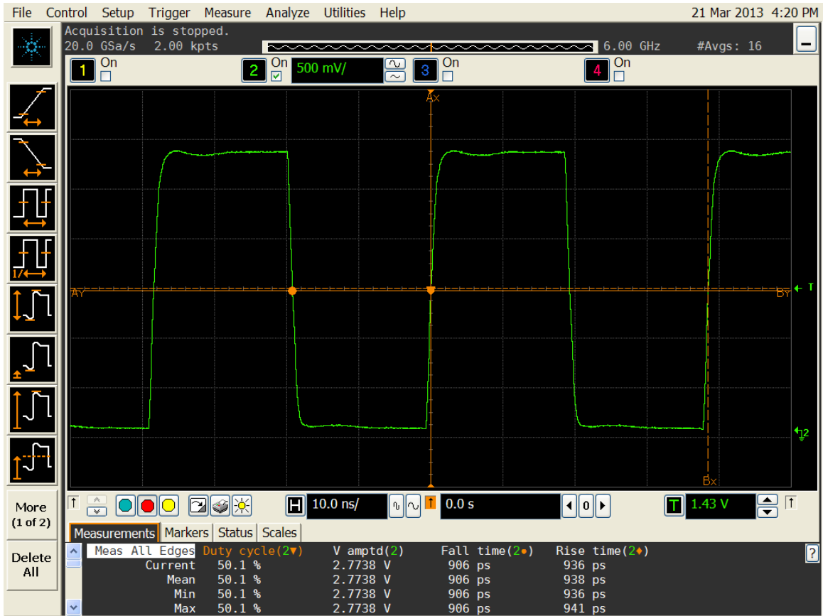
Figure 3. Duty cycle, Rise/Fall time and Amplitude 2.8V
