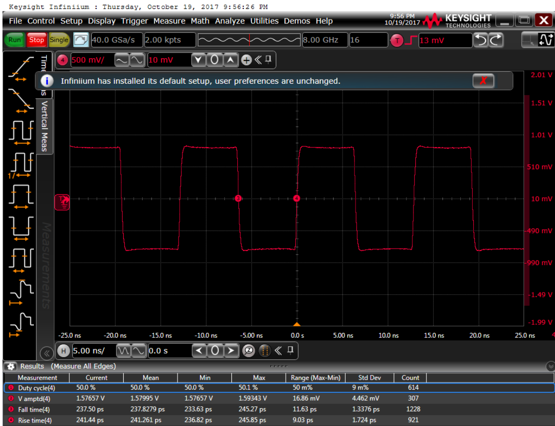
Figure 7: Output waveform, 3.3 V
