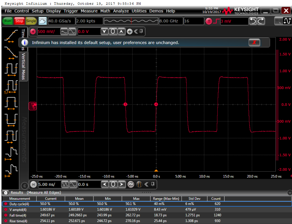
Figure 6: Output waveform, 2.5 V
