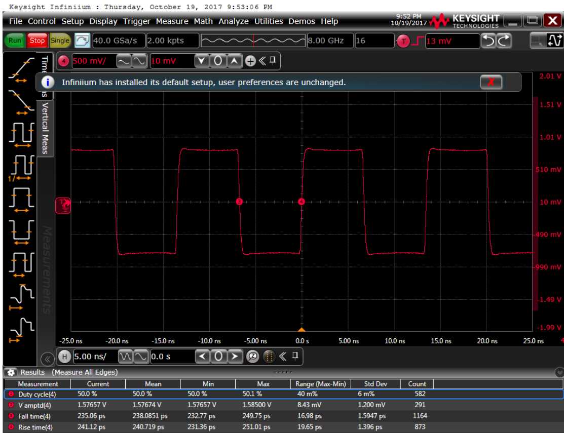
Figure 7: Output waveform, 3.3 V
