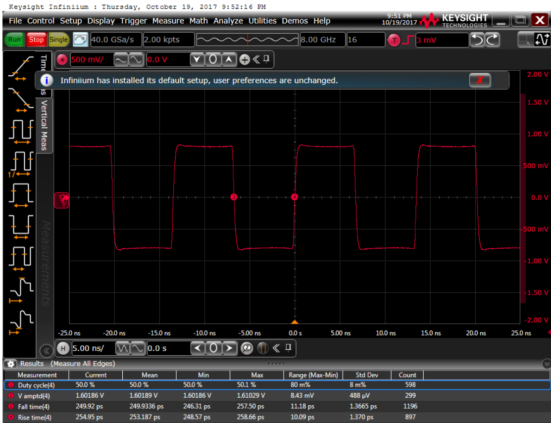
Figure 6: Output waveform, 2.5 V
