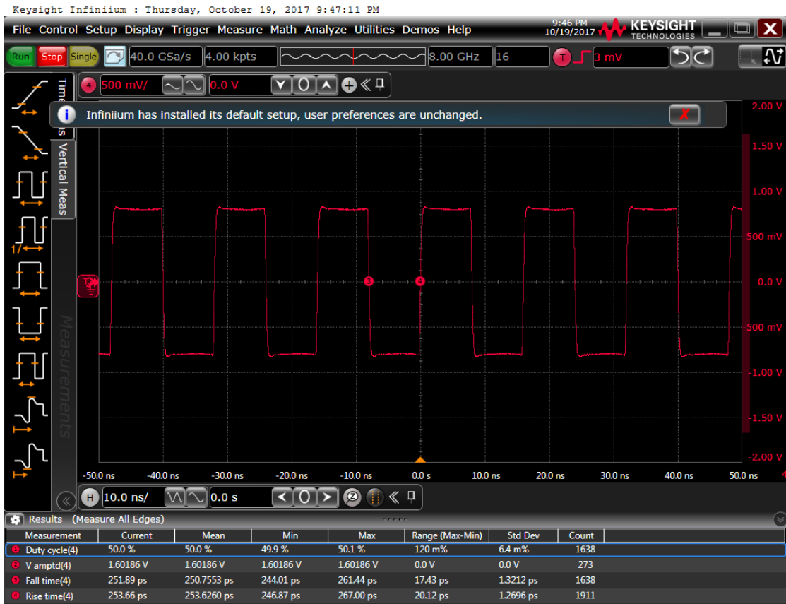
Figure 6: Output waveform, 2.5 V
