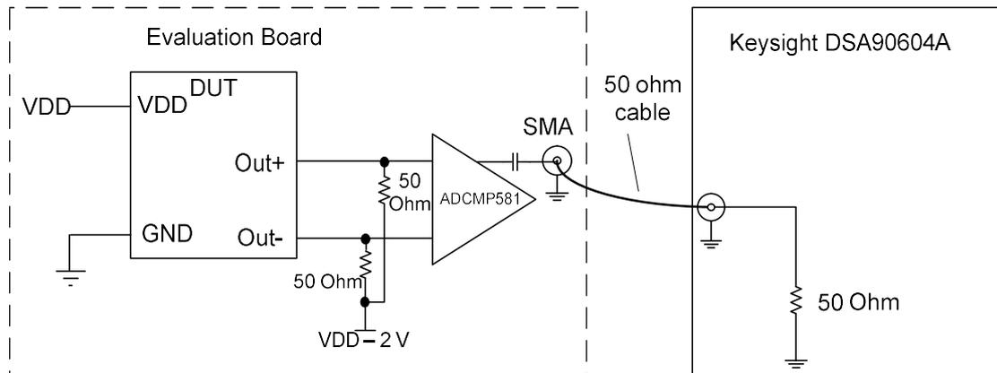
Figure 2: Test setup for measuring period jitter
