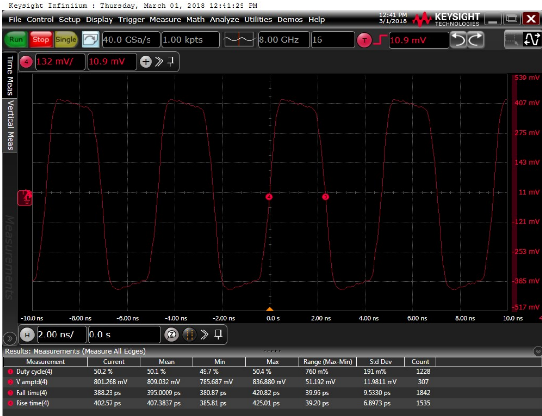
Figure 7: Output waveform, 3.3 V
