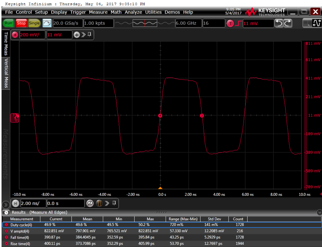
Figure 7: Output waveform, 3.3 V
