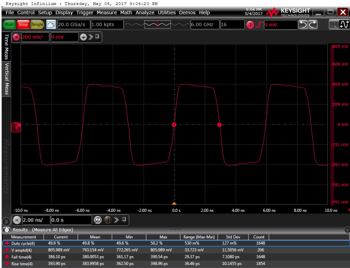
Figure 6: Output waveform, 2.5 V
