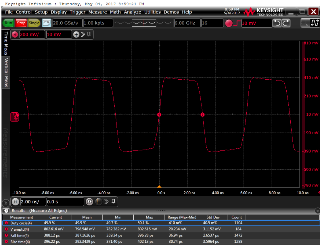
Figure 6: Output waveform, 2.5 V
