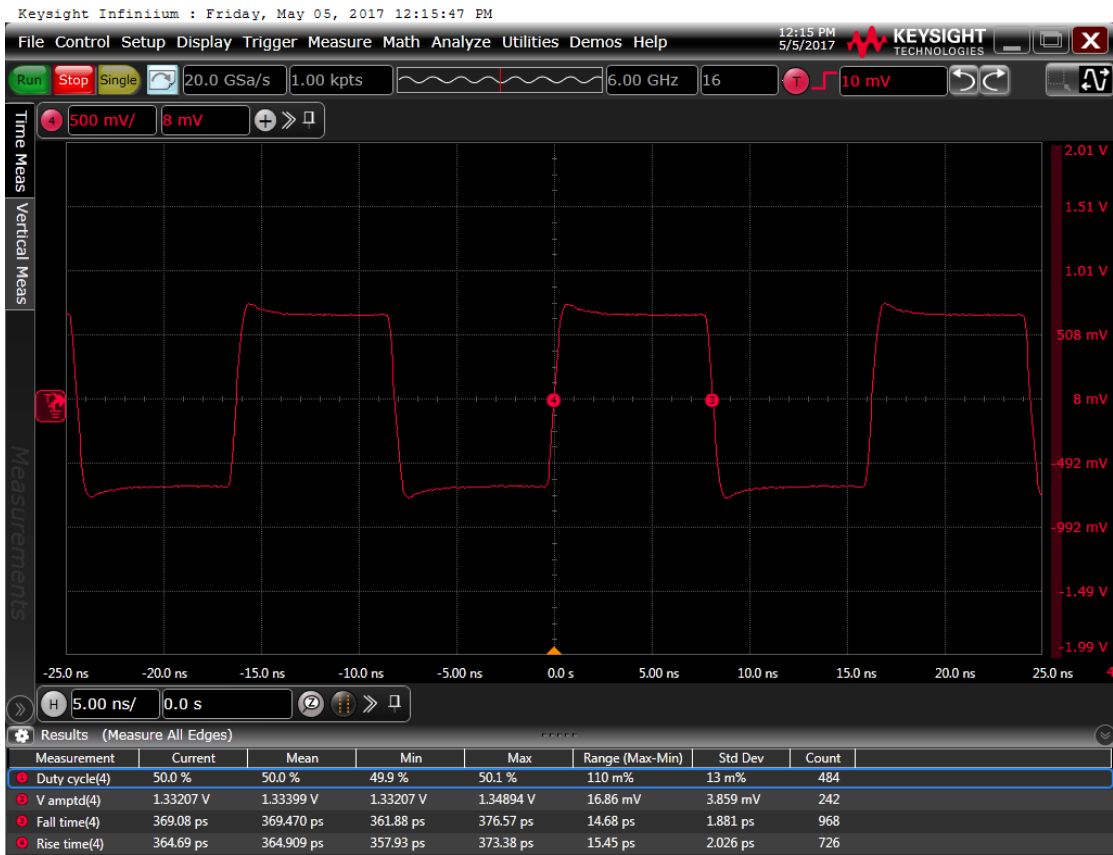
Figure 6: Output waveform, 2.5 V
