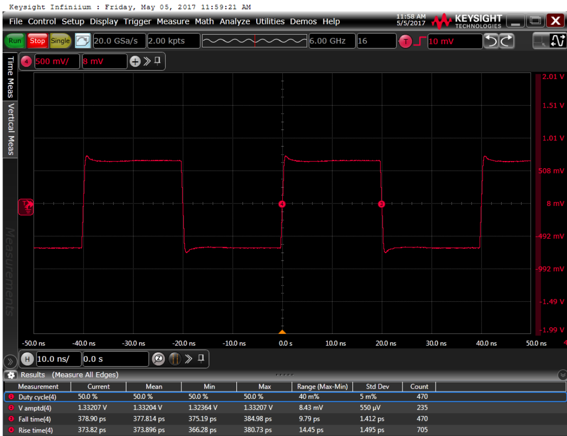
Figure 6: Output waveform, 2.5 V
