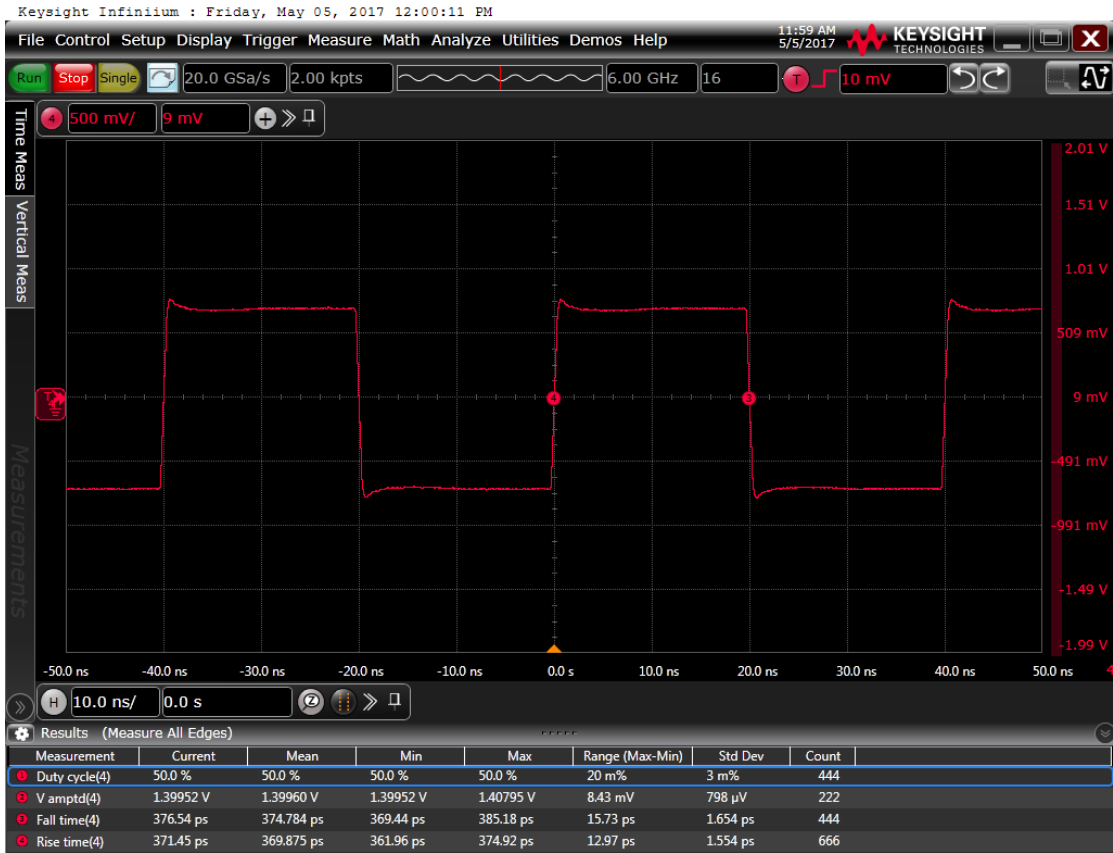
Figure 7: Output waveform, 3.3 V
