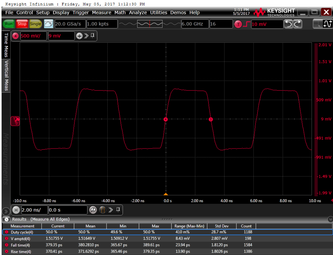
Figure 7: Output waveform, 3.3 V
