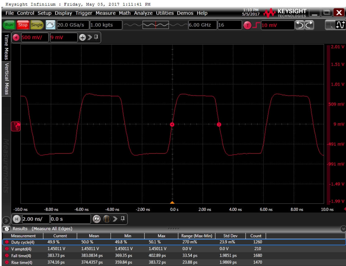
Figure 6: Output waveform, 2.5 V
