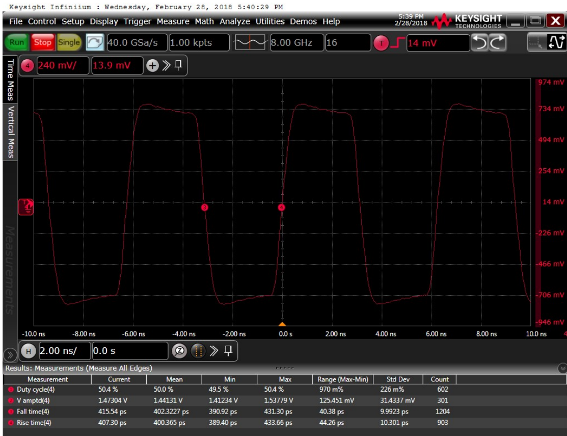
Figure 6: Output waveform, 2.5 V
