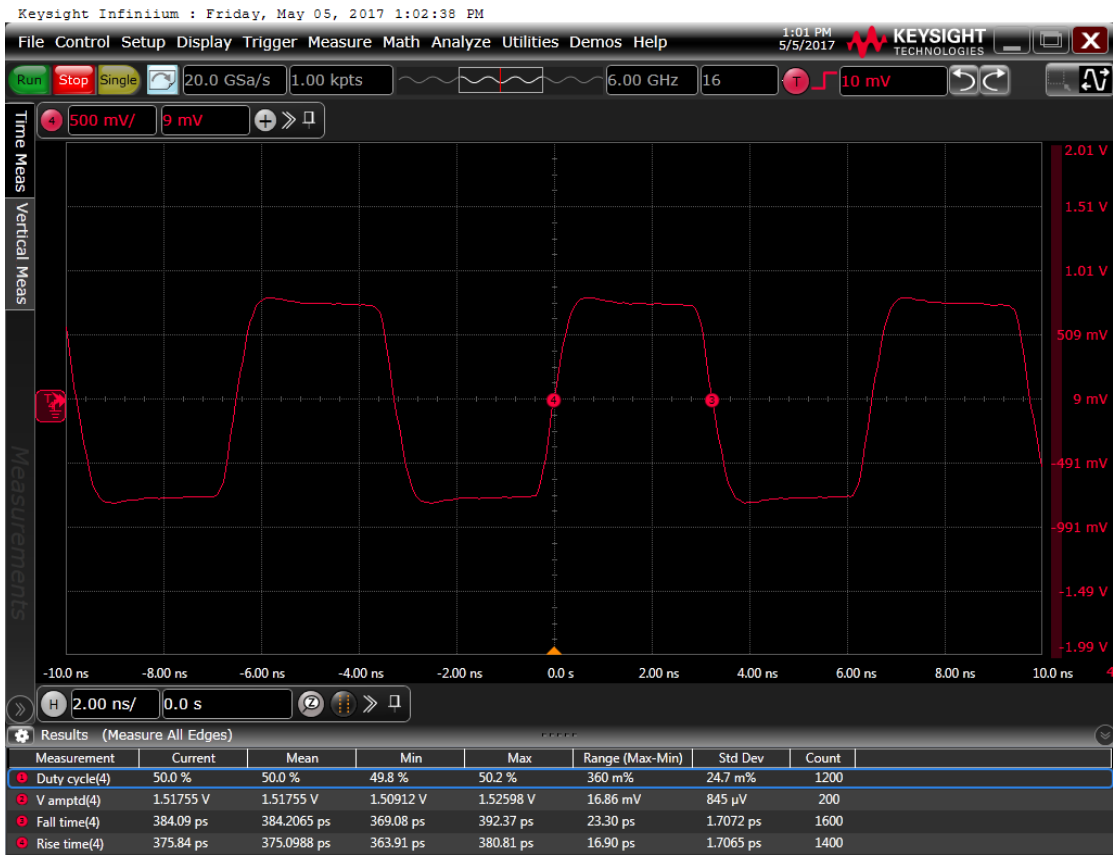
Figure 7: Output waveform, 3.3 V
