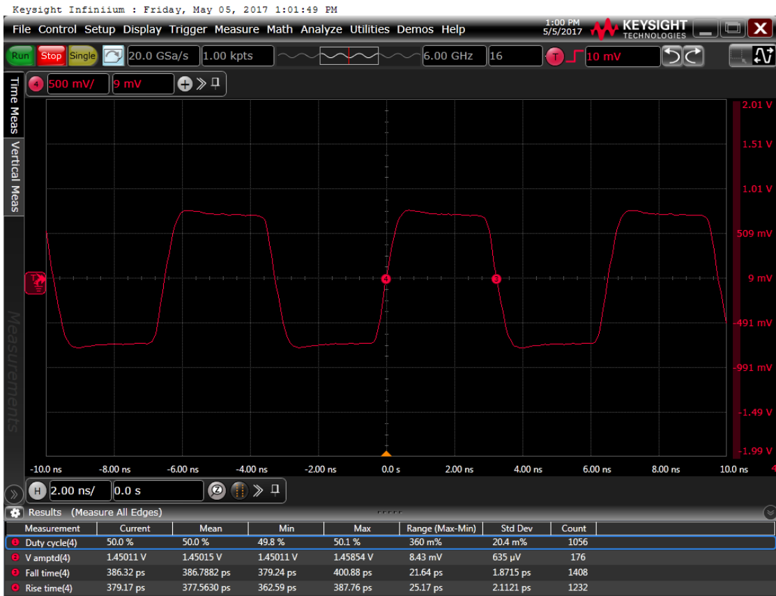
Figure 6: Output waveform, 2.5 V
