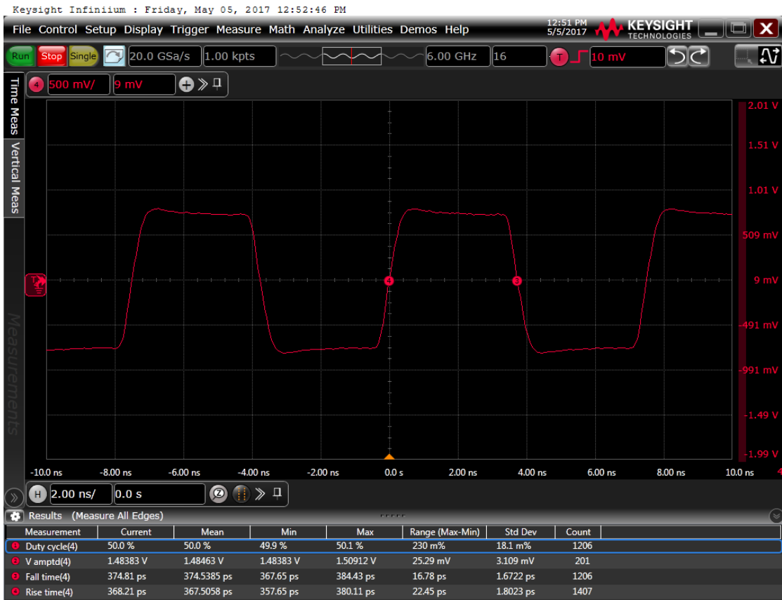
Figure 7: Output waveform, 3.3 V
