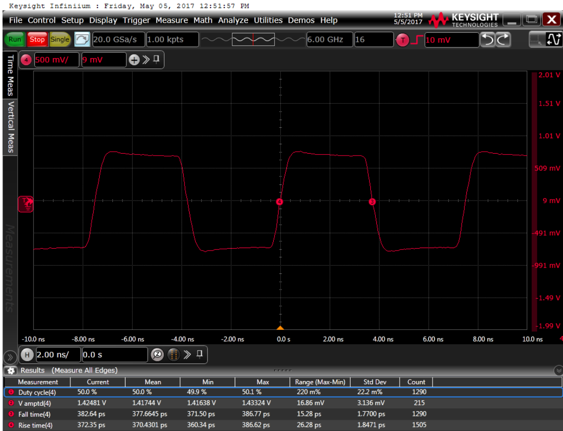
Figure 6: Output waveform, 2.5 V
