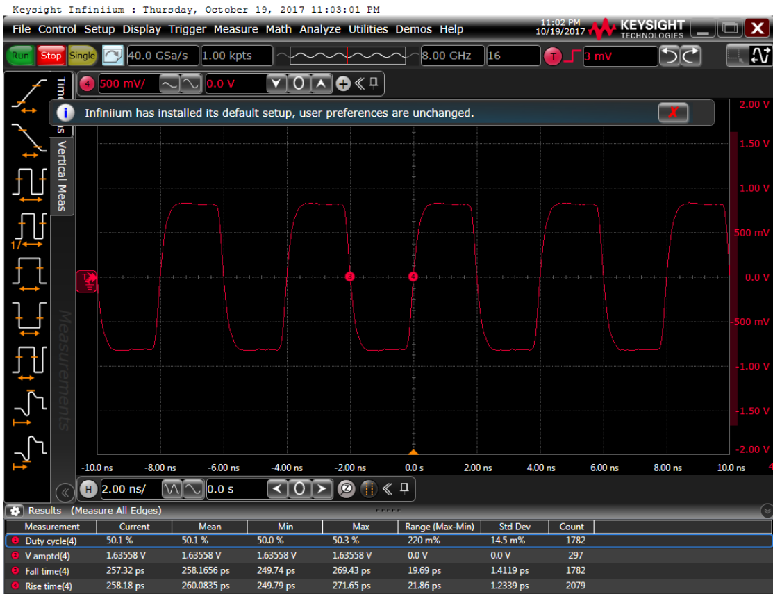
Figure 6: Output waveform, 2.5 V
