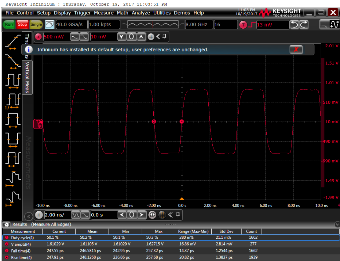
Figure 7: Output waveform, 3.3 V
