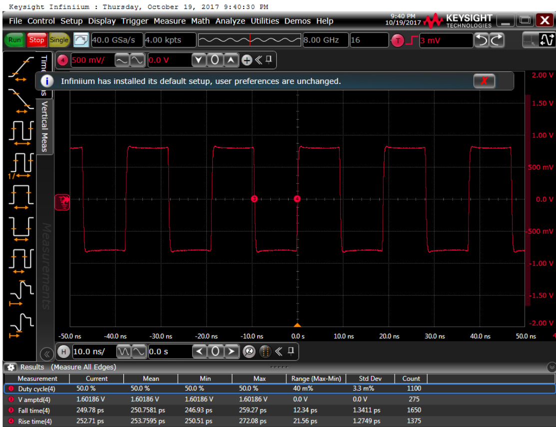
Figure 6: Output waveform, 2.5 V
