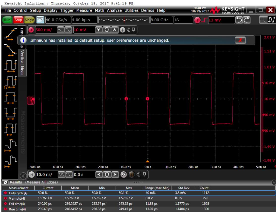
Figure 7: Output waveform, 3.3 V
