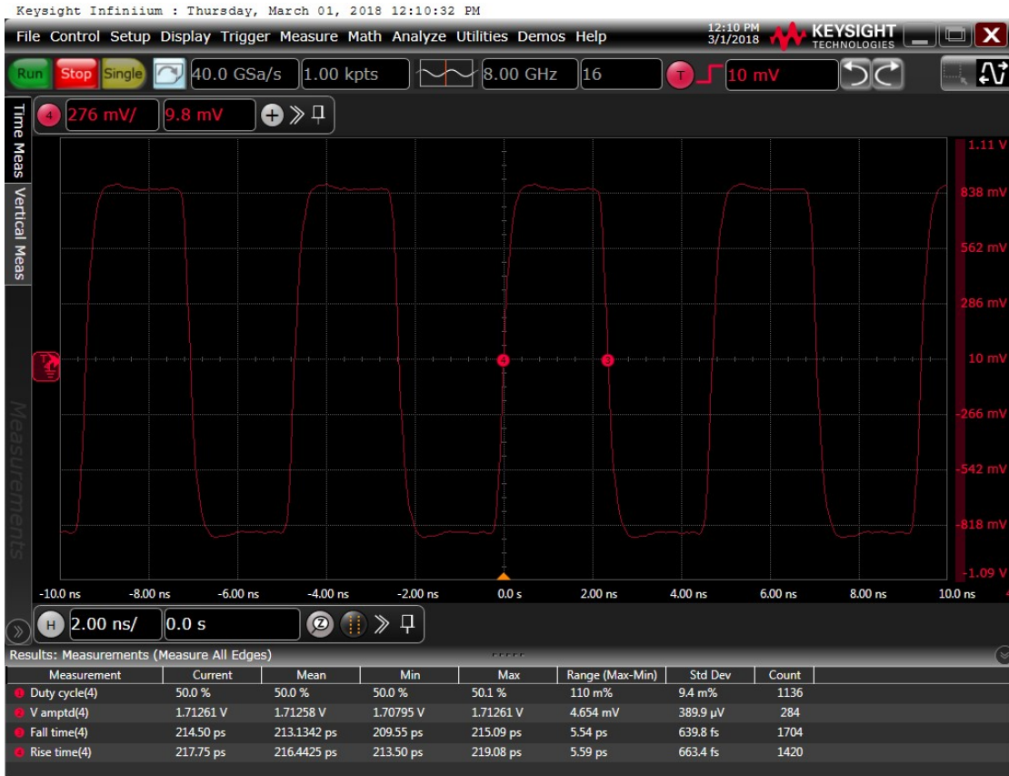
Figure 6: Output waveform, 2.5 V
