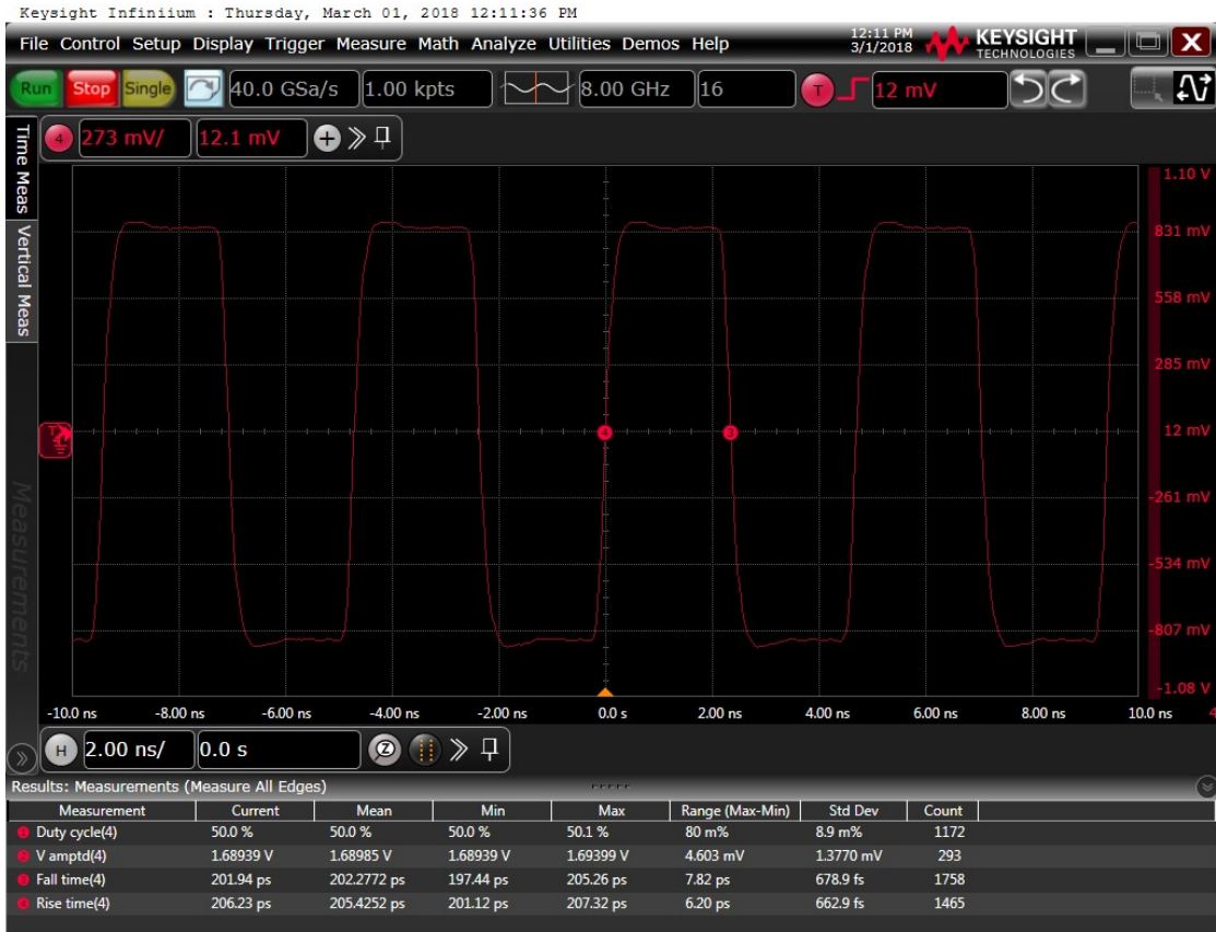
Figure 7: Output waveform, 3.3 V
