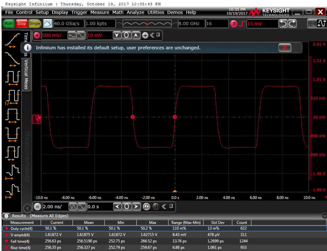
Figure 6: Output waveform, 2.5 V
