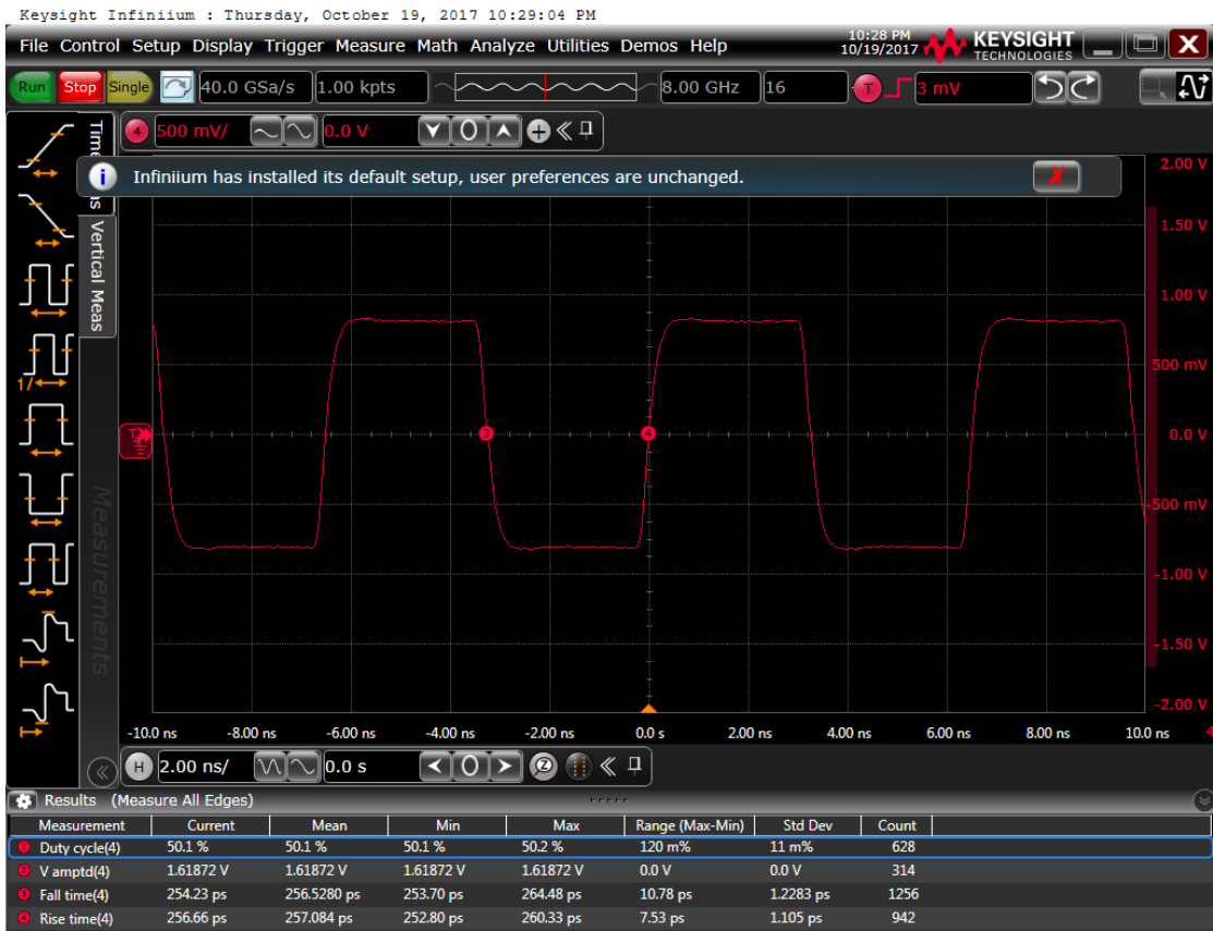
Figure 6: Output waveform, 2.5 V
