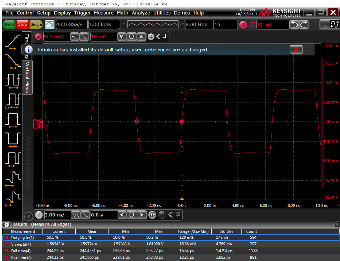
Figure 7: Output waveform, 3.3 V
