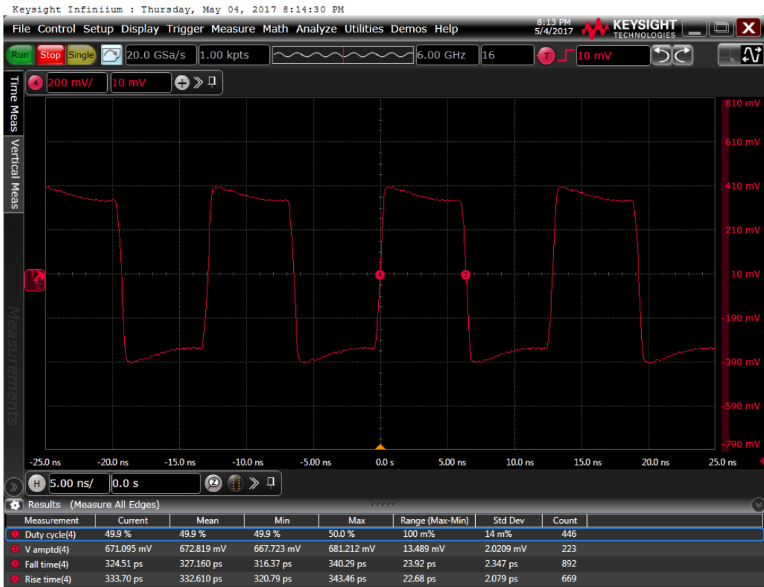
Figure 6: Output waveform, 2.5 V
