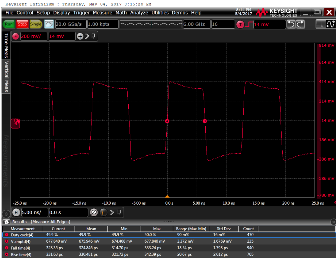
Figure 7: Output waveform, 3.3 V
