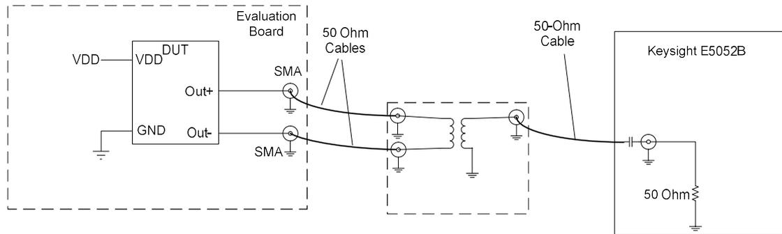
Figure 3: Test setup for measuring phase noise.
