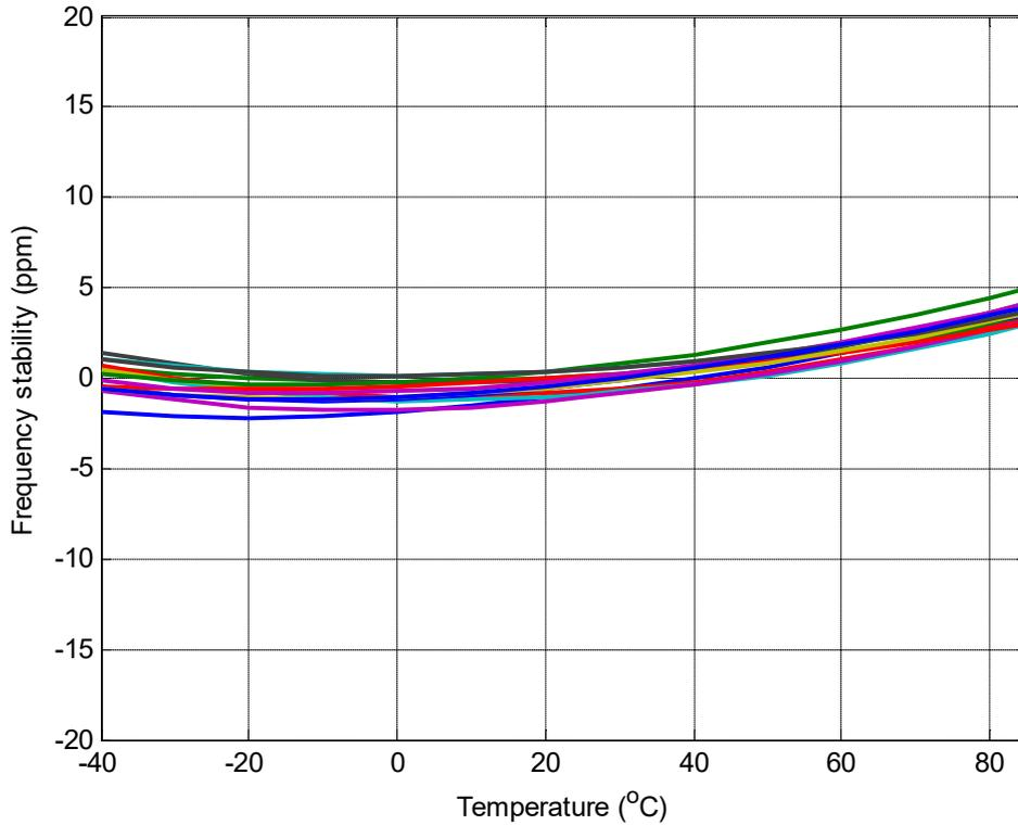
Figure 8: Frequency stability\* over temperature, 2.5 V
