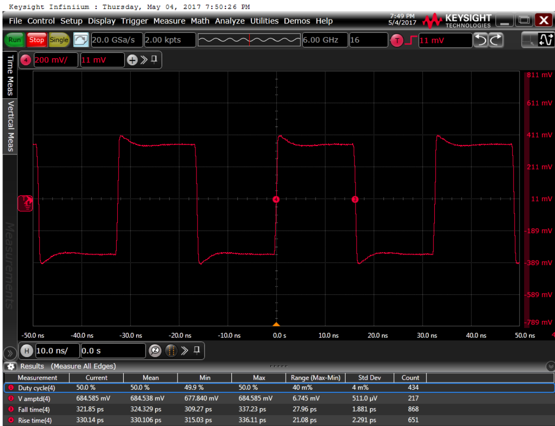
Figure 7: Output waveform, 3.3 V
