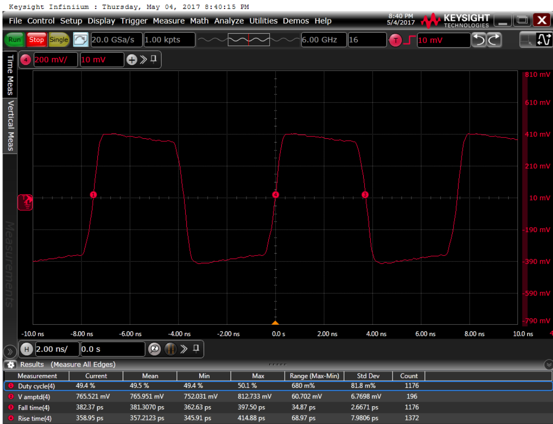
Figure 7: Output waveform, 3.3 V
