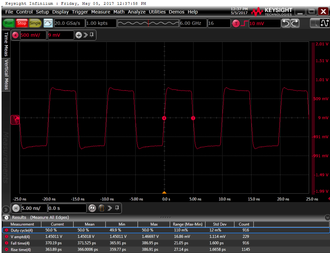
Figure 7: Output waveform, 3.3 V
