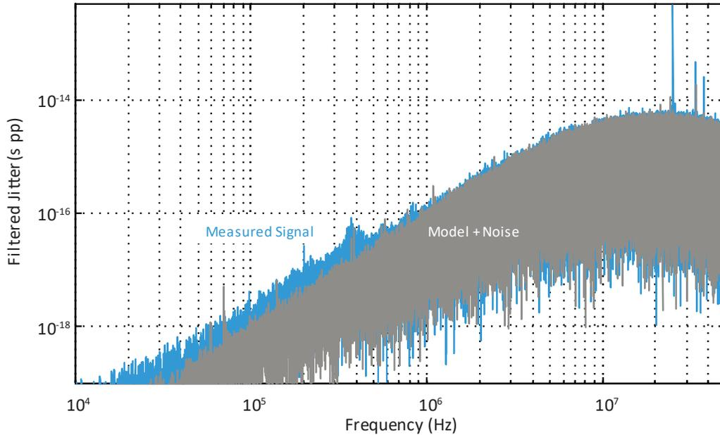
**Figure 2: Filtered jitter spectrums for (1) the signal as measured (blue), and (2) an empirical model of an ideal (jitter free) signal with noise added from the test environment (gray)**
