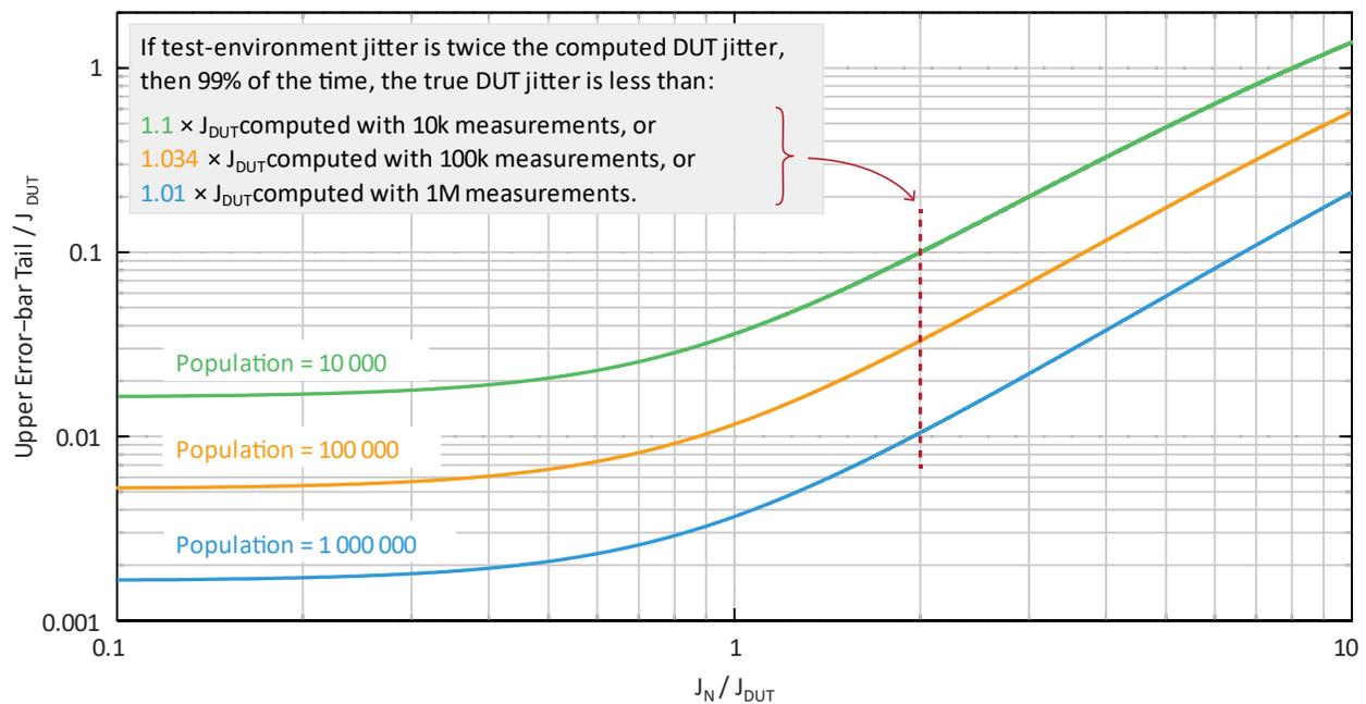
Figure 5: 98% error bars for  $J_{DUT}$  can be made insignificant with proper choice of population
