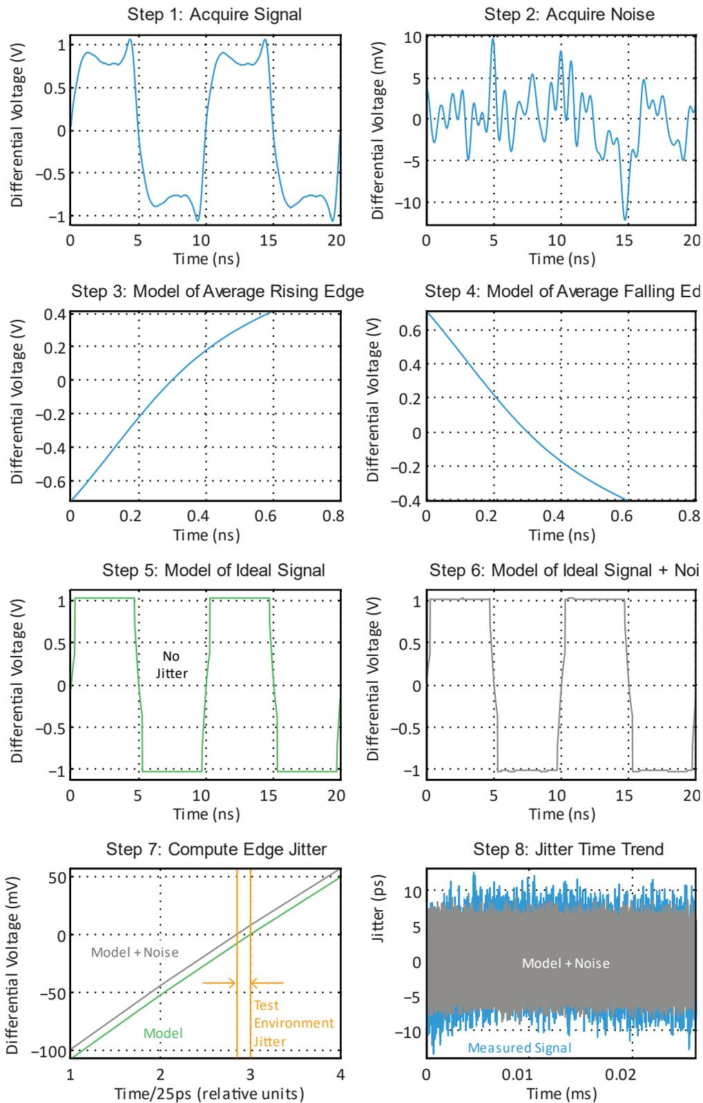
Figure 1: Illustration of key steps to remove environment noise from oscilloscope jitter data
