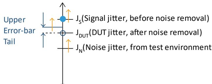
Figure 4: With  $J_{DUT}$  fixed, increasing  $J_N$  causes the upper error bar (and  $J_S$ ) to increase
