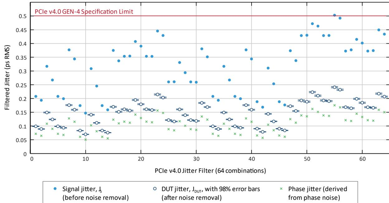
**Figure 3: Computed PCIe v4.0 GEN-4 jitter results, comparing before (●) versus after (○) noise removal, for all required filter combinations. For reference, phase jitter (×) is also shown**
