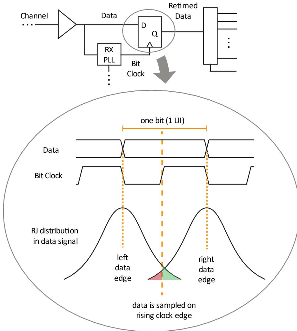
**Figure 2.1: Analysis of bit errors due to RJ in an example serial-link receiver**
