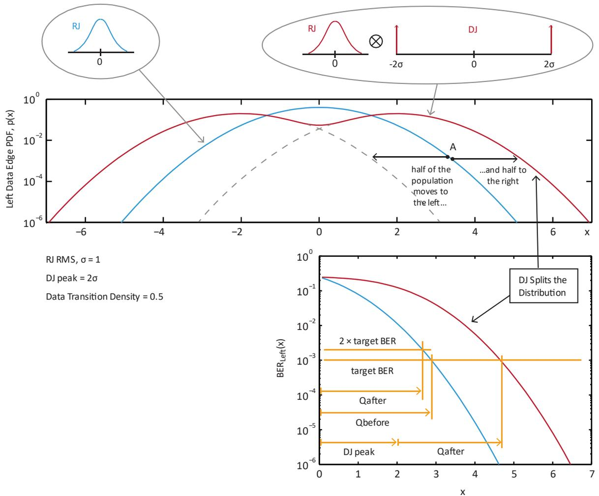
**Figure 3.1: Plots of PDF(x) (top graph) and  $BER_{Left}(x)$  (bottom graph) for a RJ distribution (blue curves) and a distribution resulting from the convolution of RJ and DJ that splits the original distribution into two halves in which only the near one effects the error rate (red curves). The mean location of the left data edge is at  $x = 0$  in the above plots.**
