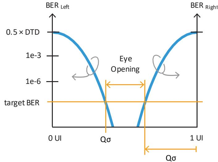
**Figure 2.3: Bathtub curve created by plotting curves for  $BER_{Left}(Q)$  and  $BER_{Right}(Q)$**
