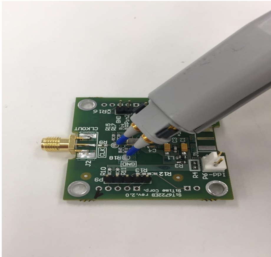
Figure 1. Proper Waveform capturing on SiT6722EB
