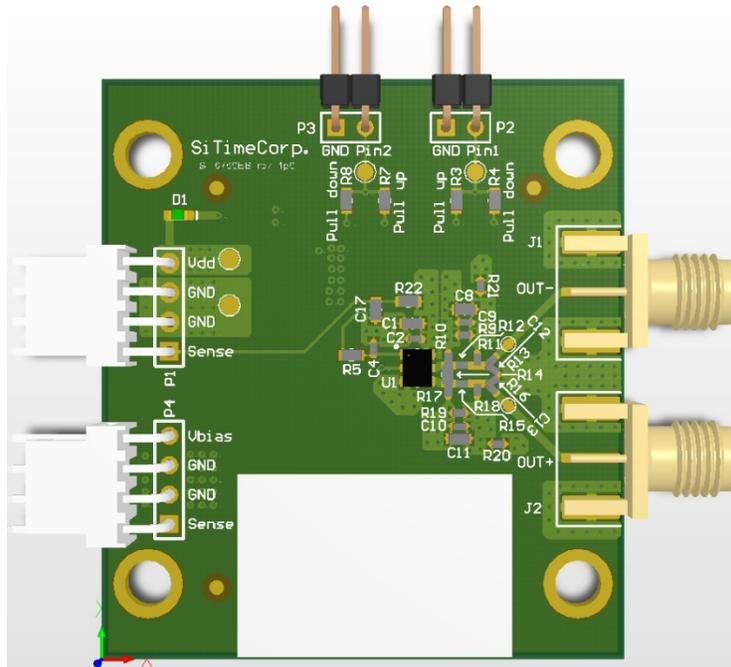
Figure 8: SiT6760EB rev 1.0 – Top view
