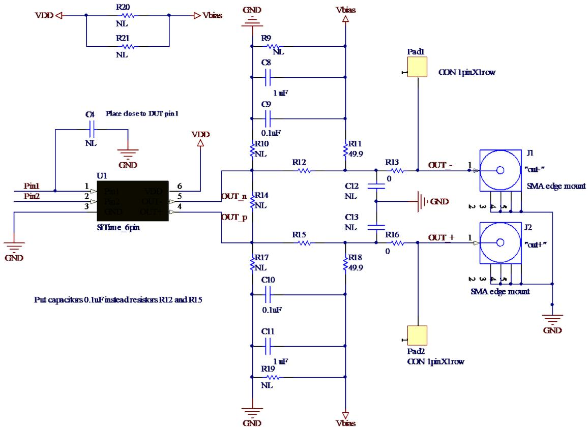
**Figure 3: Schematic of LVPECL, FlexSwing and LVDS standard shipping configuration. NL designates components that should not be loaded. Note that resistor footprints R12 and R15 should be loaded with 0.1-uF capacitors**
